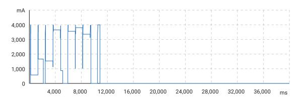
Short circuit detected. PCB is malfunctioning. Suggestion: locate 5V/12V TVS diodes on the PCB; check them and replace if damaged.
